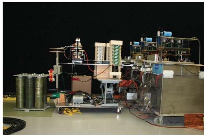
Figure 3. High peak current test stand with inductive load.
