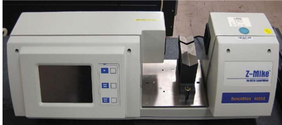
Figure 2. The Z-Mike measurement instrument, which uses a laser to measure diameters and lengths.
