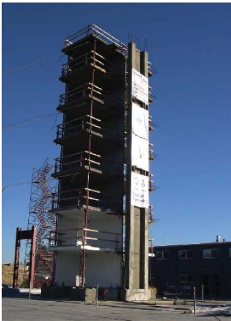
Figure 1. Seven-story structure on shake table.
