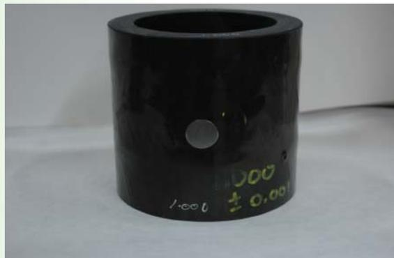
Figure 1. Fiber composite compression cylinder with 1.0-in.-diameter pin.
