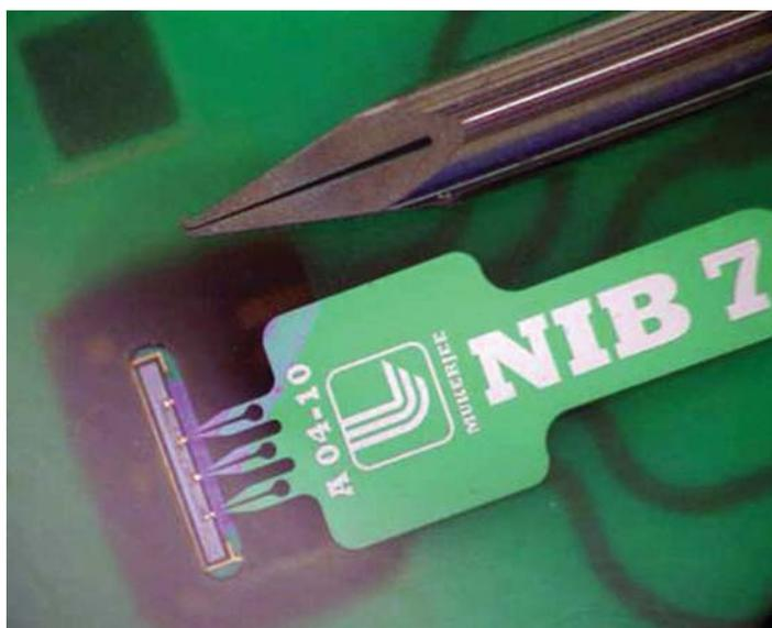
Figure 5. Demonstration of 1-to-1 registering of nib elements with micro-cantilevers and size comparison with current stainless steel nib structure.
