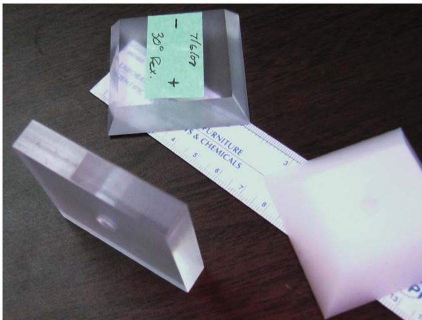
**Figure 2.** Photograph of insulators (clear HDPE, milky Rexolite ©). The HDPE insulator on its edge displays a rectangular damaged area from the UV laser beam.
