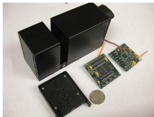
Figure 3. Complete PCR system with control electronics used to test the PCR module.
