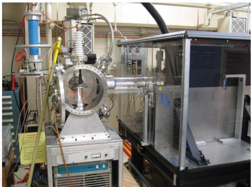
Figure 1. Photograph of the experimental apparatus with an opened cylindrical vacuum test chamber.
