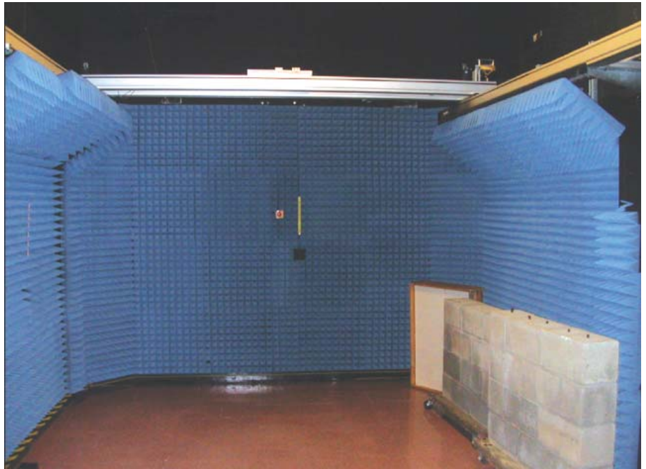
Figure 2. UWB testbed built to produce a partial anechoic effect.
