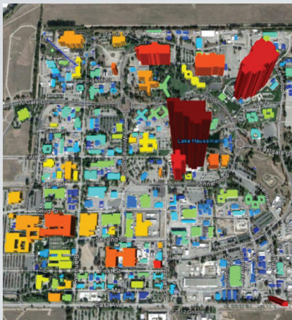
Figure 1. Google Earth rendering of GridLab D model showing site power use at Site 200.
