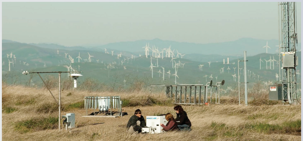
Figure 2. Field data acquisition is a critical aspect of the research for validation of forecasts. We are collecting atmospheric data and turbine performance data (Site 300 shown).
