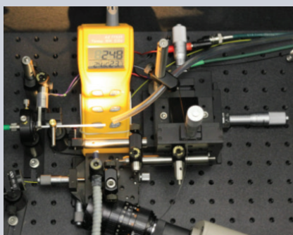
Figure 1. The experimental test setup in the gas enclosure. This benchtop setup was used to characterize different system designs to produce a successful PAS system.
