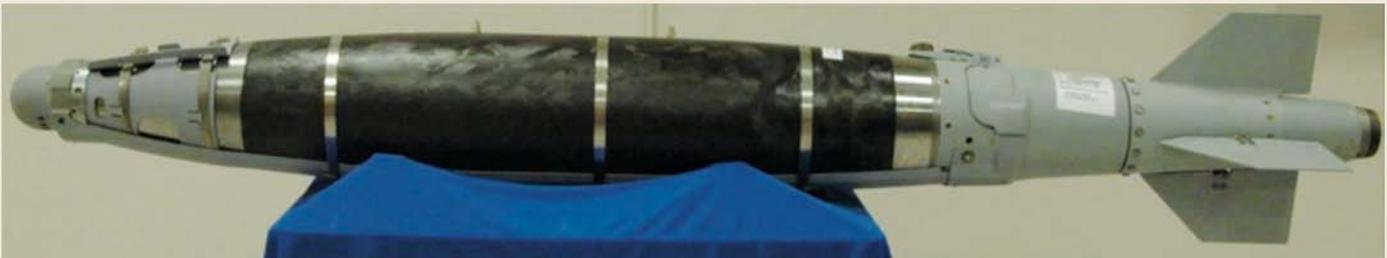
Figure 1. BLU-129/B warhead with laser JDAM guidance kit.
