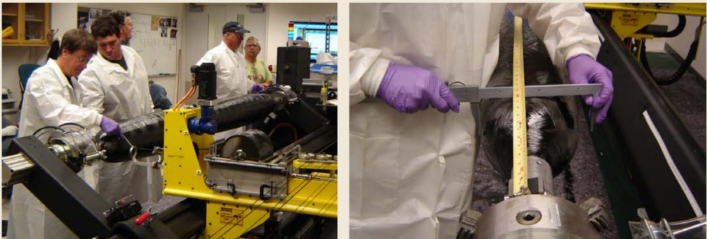
Figure 5. Case winds were carefully monitored and measured to provide consistency.
