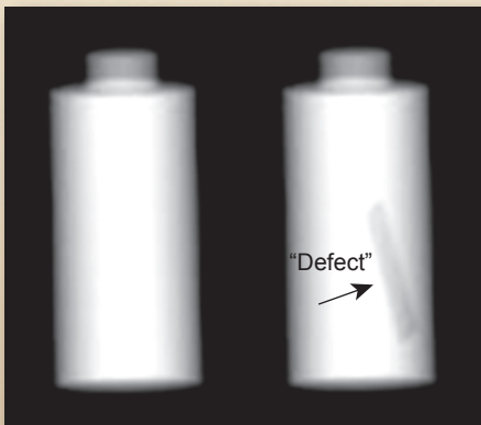
Figure 1. Simulated data used in model-based reconstruction of the proof-of-concept stacked cylinder model. The object on the left is pristine while the object on the right contains a parallelepiped “defect” which was identified and located.
