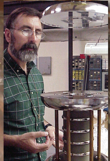
Figure 2. (Left) A conventional ~10-m-scale 7-MV DC accelerator. (Right) The Compact Directional Neutron Source seeks to achieve similar voltages at the ~ scale to enable portable operation. A test accelerator column utilizing LLNL advanced high-gradient insulator technology designed for MV potential is being assembled.
