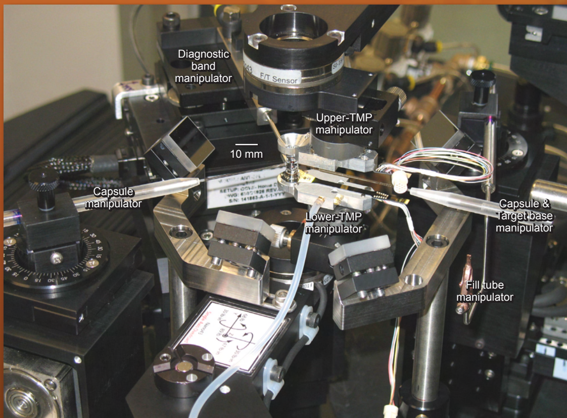
Figure 3. Close-up view of the manipulator system, with a target being assembled.
