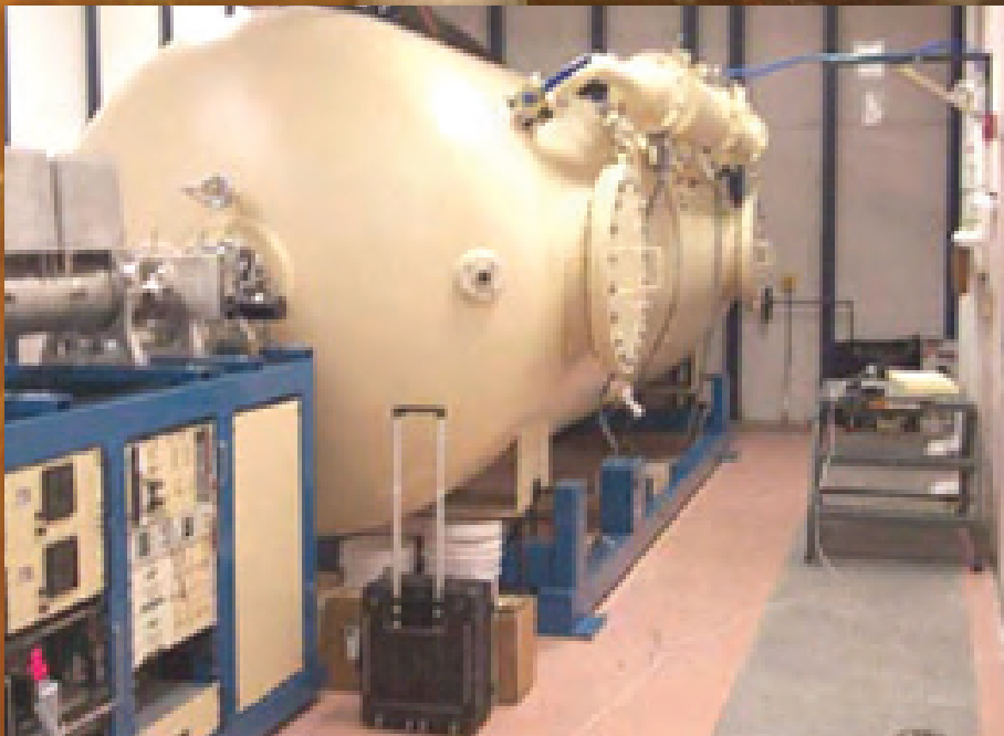
Figure 2. (Left) A conventional ~10-m-scale 7-MV DC accelerator. (Right) The Compact Directional Neutron Source seeks to achieve similar voltages at the ~ scale to enable portable operation. A test accelerator column utilizing LLNL advanced high-gradient insulator technology designed for MV potential is being assembled.
