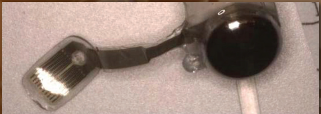
Figure 3. An overview of the 200+ electrode Artificial Retina implant. The thin-film electrode array is at the left end of the device, and the biocompatible electronics package is at the right.
