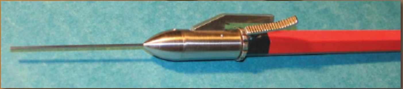
Figure 5. Overview of the new ocular surgical tool required for retinal prosthesis removal and replacement. This ocular surgical tool is designed to fit onto a standard surgical handle.
