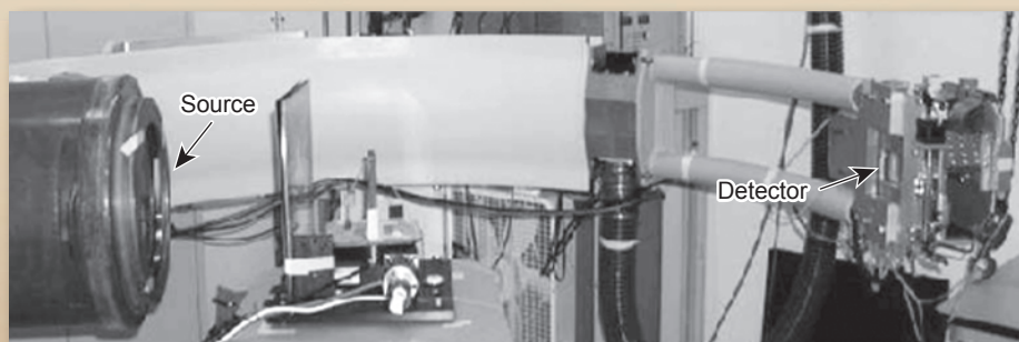
Figure 3. Photograph of the x-ray array source and array detector system designed and developed by industrial collaborator Triple Ring. (Photo courtesy of Triple Ring)
