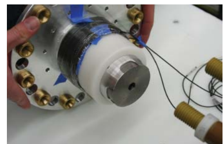
Figure 2. FRD sensor fiber installed on the ALE3D coaxial load test bed.
