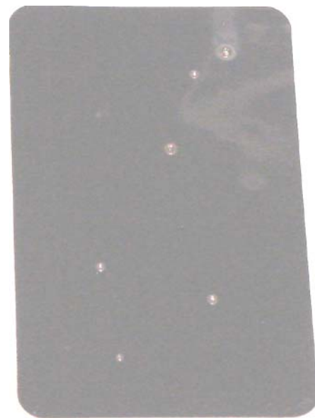
Figure 3. IR "burn" spots showing desired beam deposition energy profiles.
