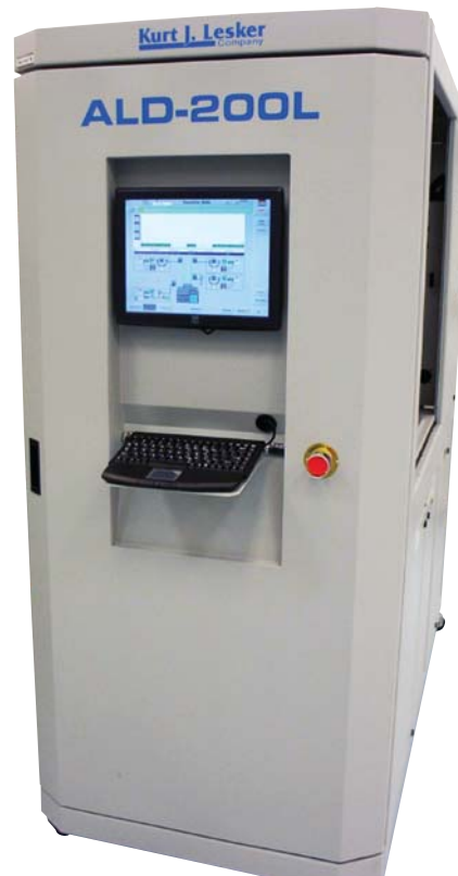
Figure 1. Atomic layer deposition tool installed in LLNL's Microfabrication Facility.
