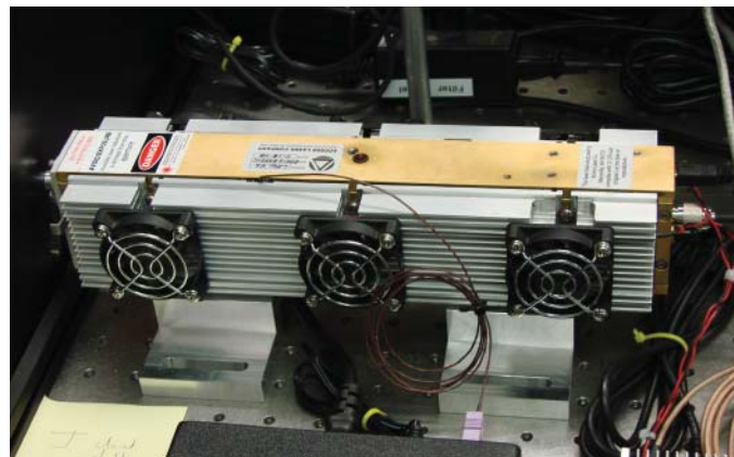
Figure 2. The 10.6- \mu\text{m} CO 2 CW laser powering DRACULA.
