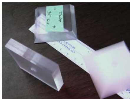
Figure 2. Photograph of insulators (clear HDPE, milky Rexolite).
