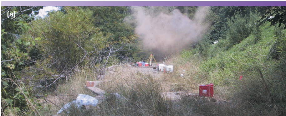
(a) Surface seismic shot detonation at the Lake Lynn site during field experiment. (b) Map view of the surface wavefield potential calculated by E3D for (a). P-waves are magenta; S-waves are turquoise. Simulations verify that advanced signal processing methods are required to detect and image underground facilities.
