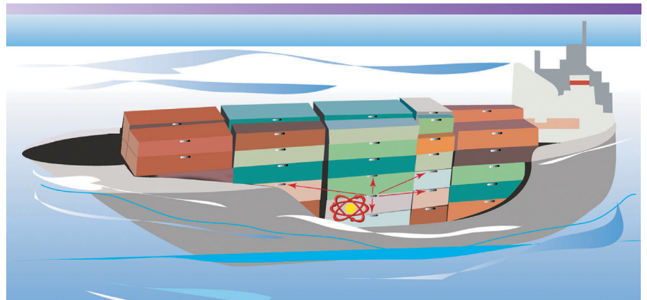
Figure 1. Conceptual drawing of a "container ship of the future" that has low-cost sensor packages in every container. Each measures the distributed radiation environment and communicates results to authorities. Clustered anomalies will trigger inspection.
