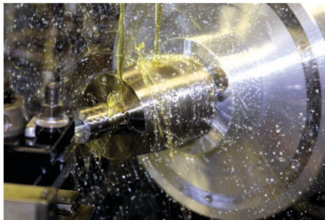
Diamond turning of the high-accuracy mandrel.
