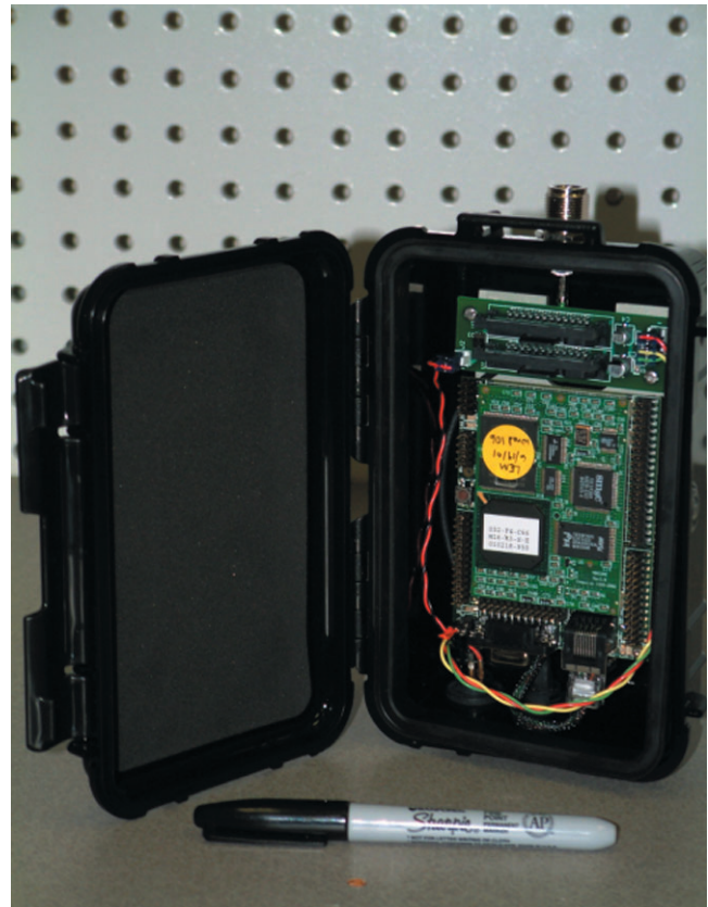
WNOD weather-tight operational node.
