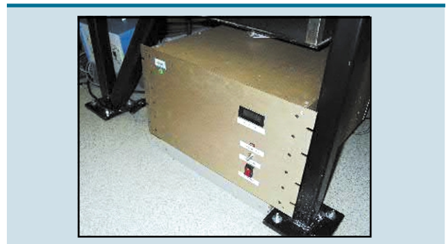
Figure 3. New completed electronics enclosure.
