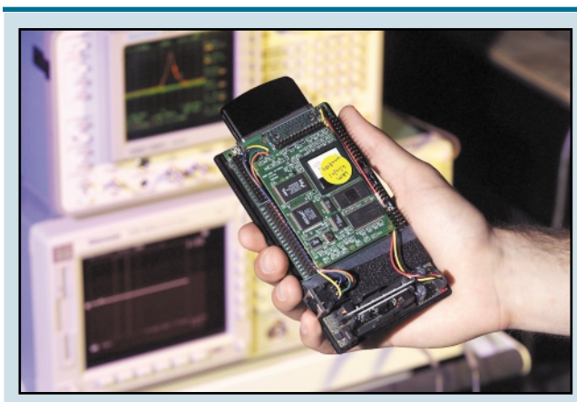
Figure 1. Wireless network node with 486 computer, wireless Ethernet, 10 Mb on-board flash memory for user applications. It is capable of creating a self-configuring, self-healing wireless network.
