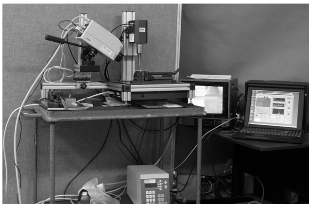
Figure 1. Photograph of the ThermoSoniX system showing IR camera, acoustic probe, test stand, PC, and monitor.
